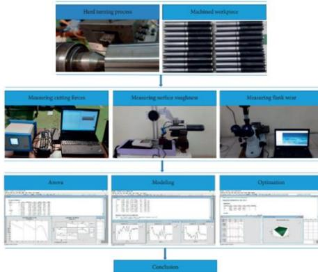
**Figure 5.9** Experimental setup diagram
