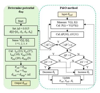
Figure 8. Algorithm flowchart of the proposed method.
