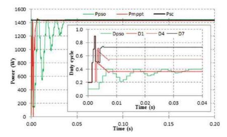
Fig. 7. Comparison of MPPT performance in No. 1
