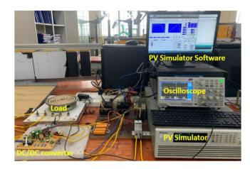
FIGURE 14 Experimental system setup.
