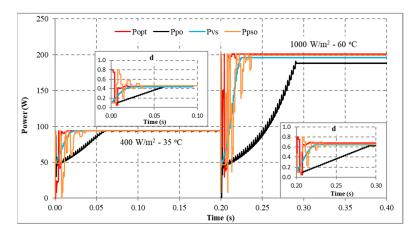
**Figure 13.** MPPT when solar irradiation and temperature increased.
