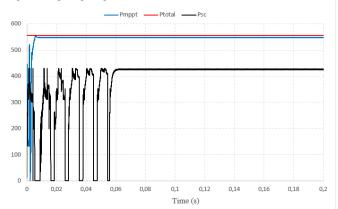
Fig. 10. Compare the speed and MPPT performance of the proposed algorithm with the PSO method (scenario 11)
