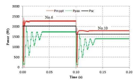
Fig. 10. Comparison of MPPT performance when changing from No. 6 to No. 10
