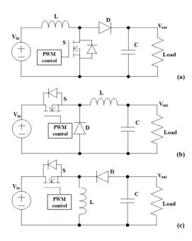
FIGURE 6 DC/DC converters: (a) Boost; (b) Buck; (c) Buck-boost.
