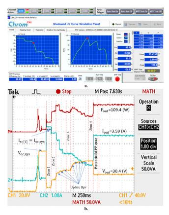
FIGURE 14. Experimental results with three parallel strings a. efficiency, and b. waveforms.
