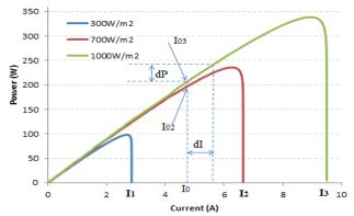
Fig. 4. Characteristic curve P-I of a PV module PV under various conditions
