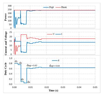
Figure 10. MPPT simulation under standard condition.
