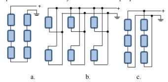
Fig. 1. Connection configurations of PV modules: a. SC, b. PC, c. SPC
