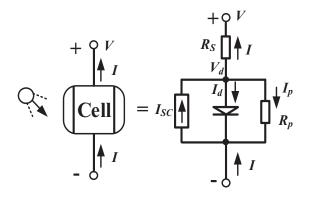
Fig. 1. PV cell equivalent circuit.
