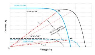
**FIGURE 7** The I(V) curves in the operating limit of PV. PV, photovoltaic.
