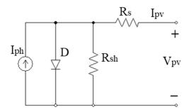
Figure 1. Equivalent circuit of PV cell.
