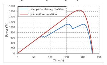
Fig. 2. P-V characteristic under different conditions.
