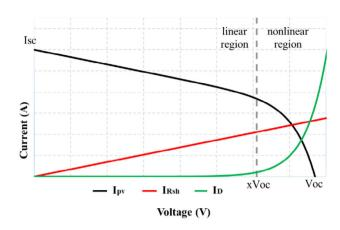
**FIGURE 8** Working regions of PV module characteristic curves. PV, photovoltaic.
