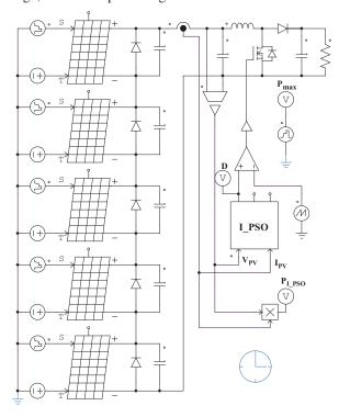
Fig. 5. Simulation model of the proposed system
