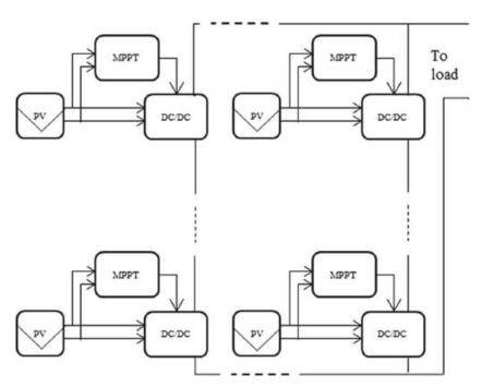
Fig. 4. Proposed solution structure
