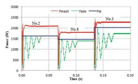
Fig. 11. Comparison of MPPT performance under continuous change
