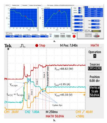
FIGURE 12. Experiment MPPT for No.02 with a. efficiency, and b. waveforms.
