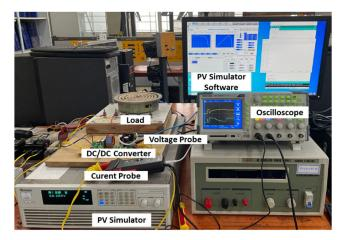
FIGURE 10. Experimental system setup.
