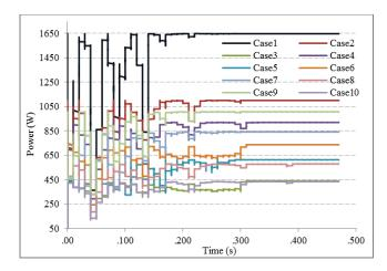
Fig. 7. Measured PV power waveforms under MPPT process.
