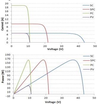
Fig. 2. Characteristic curves I-V and P-V of various configurations in identical operating conditions
