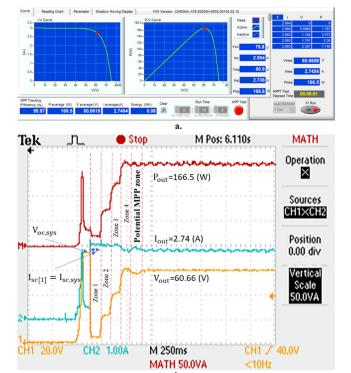
FIGURE 11. Experiment MPPT for No.01 with a. efficiency, and b. waveforms.
