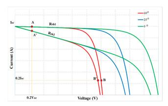
Figure 4. The I(V) characteristics under different conditions of temperature and R<sub>sh</sub>.
