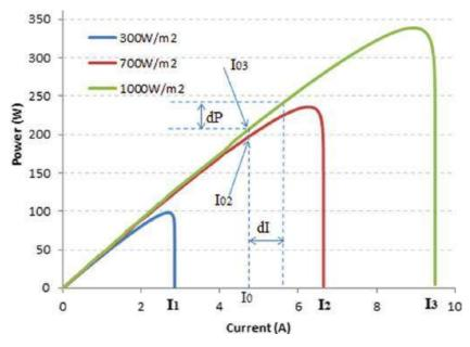
Fig. 3. P-I characteristics of PV module under different conditions
