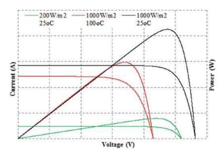
Fig. 2. Effect of radiation and temperature on the P–V and I–V curves
