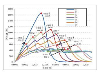
Fig. 3. GMPP under partial shading conditions
