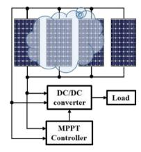
**FIGURE 4** Schematic diagram of the PV control system in this research. PV, photovoltaic.
