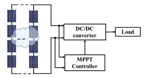
FIGURE 1. Schematic diagram of the proposed PV system.
