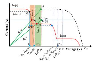
FIGURE 2. Determine MPPs on the I-V curve under PSC.
