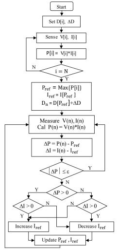
Fig. 6. Proposed algorithm flowchart
