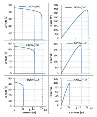
Fig. 3. Characteristic curves V-I, P-I as solar radiation levels vary
