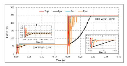
Figure 16. MPPT under the operating conditions from No. 01 to No. 05.
