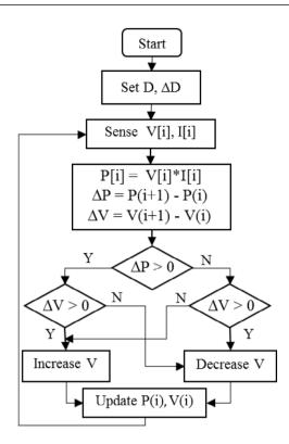
**FIGURE 3** Flowchart of conventional P&O algorithm. P&O, perturb and observe.
