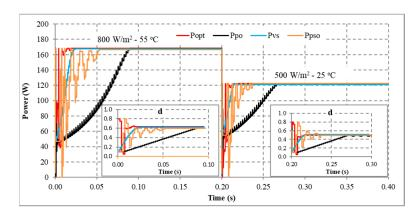
Figure 14. MPPT when solar irradiation and temperature decreased.
