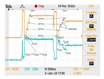
FIGURE 13. Experiment with MPPT under variable conditions.
