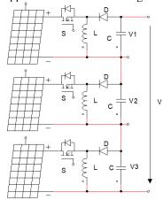
Fig. 5. Connection configuration of DC-DC converter
