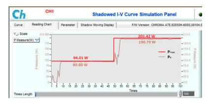
Figure 21. MPPT under the operating conditions from No. 12 to No. 09.
