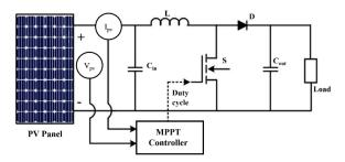
Figure 5. Schematic diagram of the PV control system in this research.
