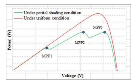
Fig. 1. P–V characteristics under operating conditions
