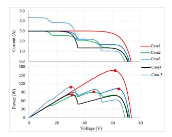
FIGURE 5. Characteristic curves of PV system under PSC.
