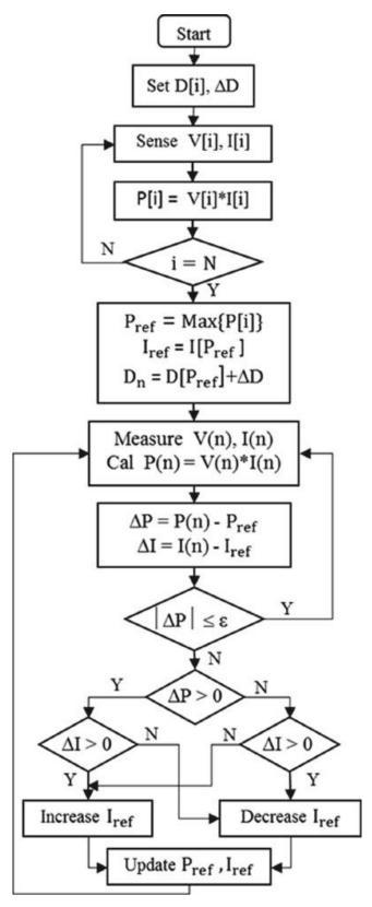
Fig. 6. Flowchart of the proposed algorithm
