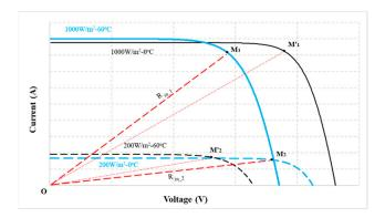
**Figure 3.** The I(V) characteristics under different working conditions.
