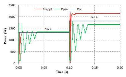
Fig. 9. Comparison of MPPT performance when changing from No. 7 to No. 4
