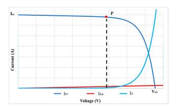
**Figure 2.** The I(V) characteristics under standard working conditions.
