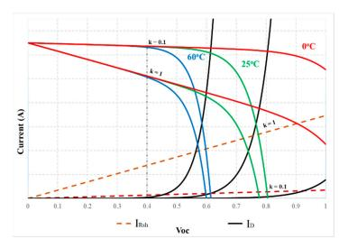
**Figure 6.** The I(V) characteristic curve of the PV module MSX-60.
